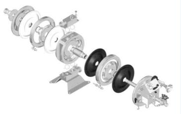
The "Guardian" rupture protection system can be fitted to all Flotronic Pumps. With this system a secondary chamber is created by an additional diaphragm behind each of the primary pump diaphragms to capture liquid upon primary diaphragm rupture. This chamber can be in low-cost Polypropylene or a material to match the pump wetted body.
